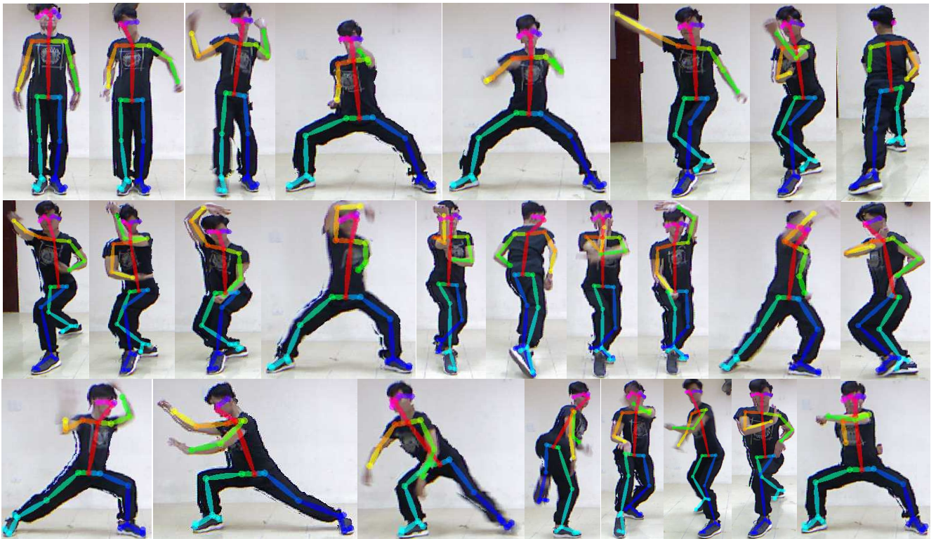
Figure 17. Estimated keypoints and joints on video frames showing a chain of martial art poses: body joints are colored red, left hand joints are colored green, right hand joints are colored yellow, left foot joints are colored blue, and right foot joints are colored cyan.
