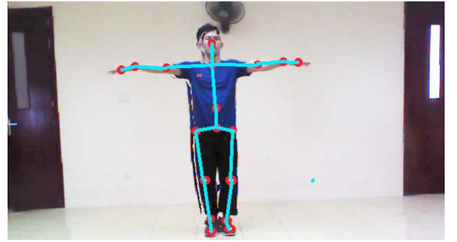
Figure 7. Illustration of the obtained image from MS Kinect sensor v1 and annotated keypoints of the skeleton model.
