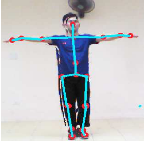
Figure 8. Illustrations on ground-truth for keypoints. Red points are keypoints on the human body. Blue segments show connections between parts of the human body.
